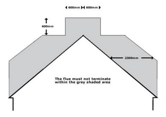
The height of the chimney or flue will be determined by the pitch of the roof. Table 2 offers an indication of the different flue and chimney stack heights necessary to give the mandatory required roof clearances when the flue or chimney exit point is beyond 600mm of the ridge.
